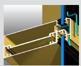
Concealed drainage designed to shed water more efficiently and improve aesthetics without runs of visible holes along the face. Very high water performance greater than 600 Pa.
