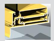
Sub-sill, sub-head and sub-jambs available. The sub-sill has additional support leg under the glass, designed to carry weight of heavy glass unit and prevent frame dishing.
